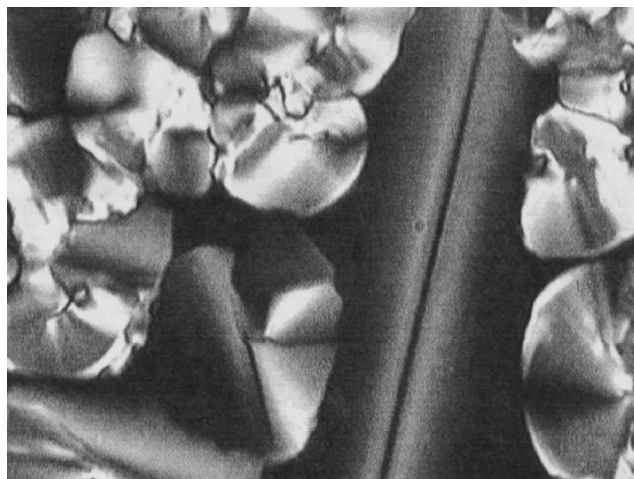
Figure 1. Typical texture between crossed polarizers after cooling without a field; grey spindle-like bâtonnets with dark straight central lines and fan shaped domains coexist. T = 23^\circ\text{C} , d = 8\ \mu\text{m} , substrates are coated with octadecyltriethoxysilane; the picture represents 0.5\ \text{mm} \times 0.3\ \text{mm} area.
